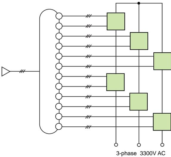
Fig. 2 Internal configuration of inverter cell
