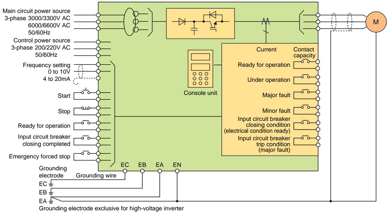
Note: Be sure to use an EA grounding electrode exclusive for the high-voltage inverter, and isolate it from the main grounding lines of other devices.
