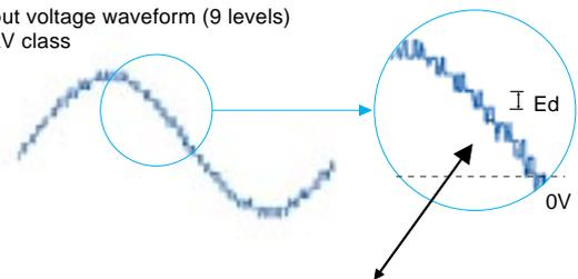
In the 3kV class Fuji Electric's medium-voltage inverter, the output voltage changes in 9 steps (corresponding to 9 levels) within 1/4 cycle. The voltage value of one step equals the DC intermediate circuit voltage  $E_d$ . Therefore, for the same voltage output, a larger number of steps means a smaller voltage value at one step. Thus, Fuji Electric's inverter can also reduce the surge voltage appearing at the motor terminal and thereby moderate the stress applied to the motor.
